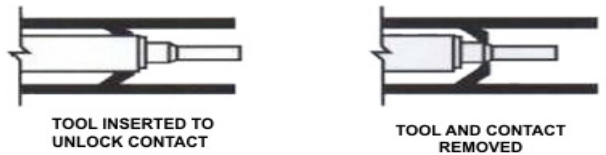
Figure 7-23. HD/HDP Unlocking Contacts
